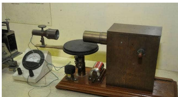
First radio prototype built by J C Bose. (Courtesy: Bose Institute)
