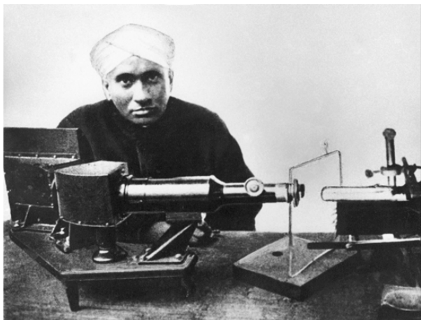
C V Raman with his Spectrograph, the first Raman Spectrum was obtained with his spectrograph in 1928. (Courtesy: Indian Academy of Sciences- C V Raman: A Pictorial Biography)
